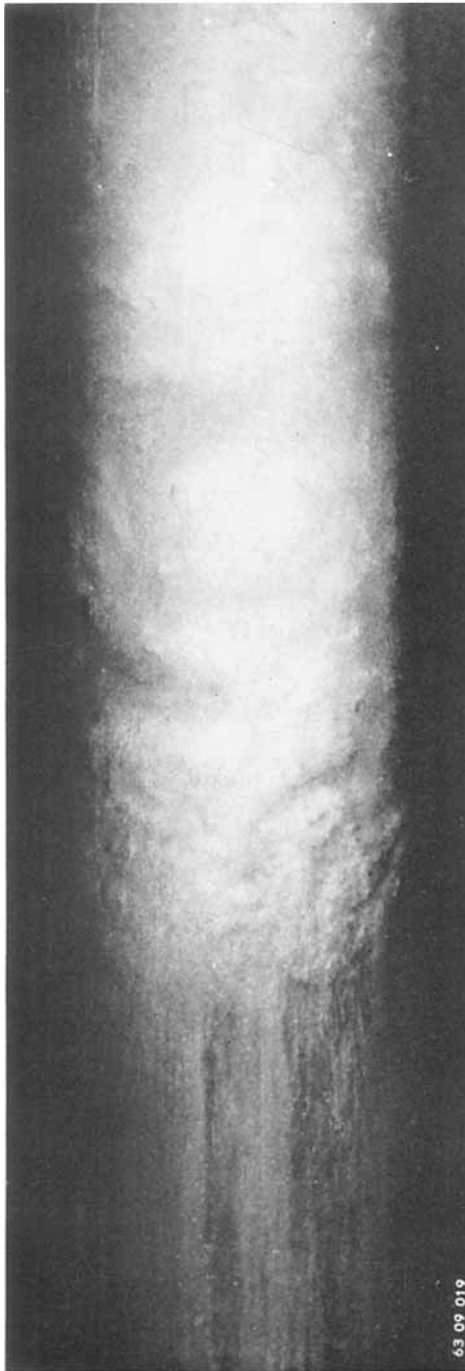
U_{t_1} = 63 \text{ m/sec} U_{m_2} = 16.5 \text{ m/sec} FIGURE 7. Mixing shock. a = 23.5 , \epsilon = 78.0 , \theta = 3.44 , \phi = 0.250 , M_t = 11.1 \text{ kg/sec} , D_n = 15 \text{ mm} . Flow from left to right. Exposure time 3 \times 10^{-6} \text{ sec} . Black velvet background.
